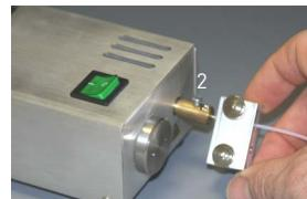
» The flange has to be cooled down fast. Press it for approx. 10 seconds onto the plain surface of the cooling plate (8) (not into the bores). The exact time has also to be defined in several trials.
