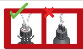
The special highlight: The body of the distributor can be turned independently from the screw cap. This means, the tubing will not be disarranged when the distributor is fixed on another bottle.
